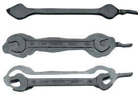
Surplus material is removed by trimming presses.
